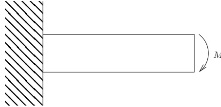
Figure 4.5: Cantilever beam in pure bending
